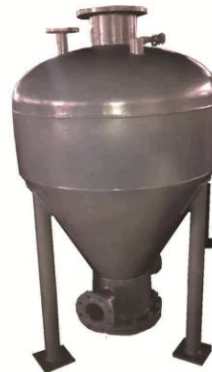
上引式仓泵 Ascending suction transport
