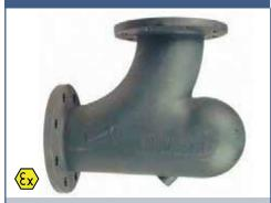
**DESIGNED FOR:** Creates a non-impact deflection zone to smoothly guide the product round the elbow unique vortex chamber eliminating or greatly reducing wear.
